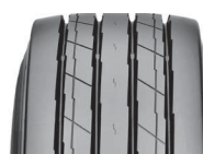
Regrooved tire (0 = Regrooving depth indicators)
